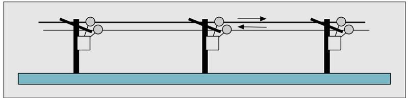
■ Figure 5. A (horizontally) balanced system using differential drive.
