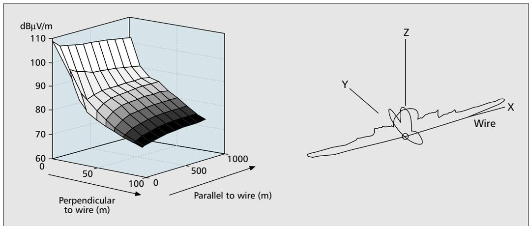
■ **Figure 4.** 20 MHz electric near-fields (left) and far-field pattern (right). The maximum far-field gain perpendicular to the wire is 22 dB below the forward peak.
