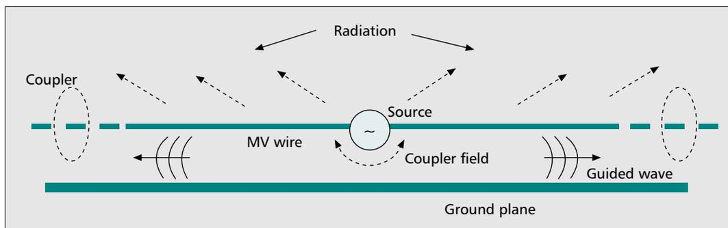
■ Figure 2. Electromagnetic model of a BPL system.
