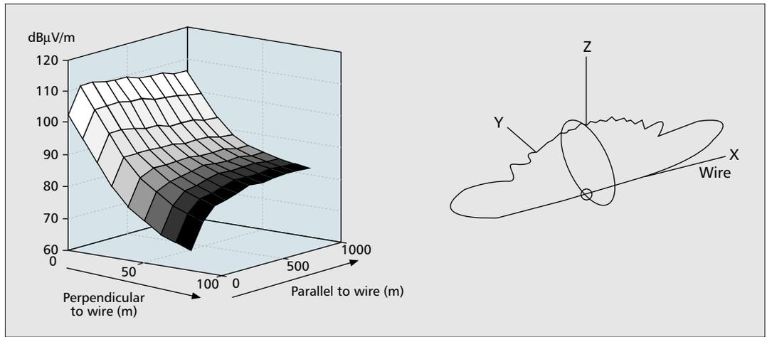
■ **Figure 3.** 2 MHz electric near-fields 2 m above street level (left) and far-field pattern (right). Indicated distances are measured at ground level from a point directly beneath the coupler. The maximum far-field gain perpendicular to the wire is 12 dB below the forward peak.
