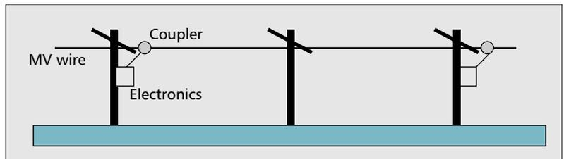
■ Figure 1. BPL system using aerial MV wires.
