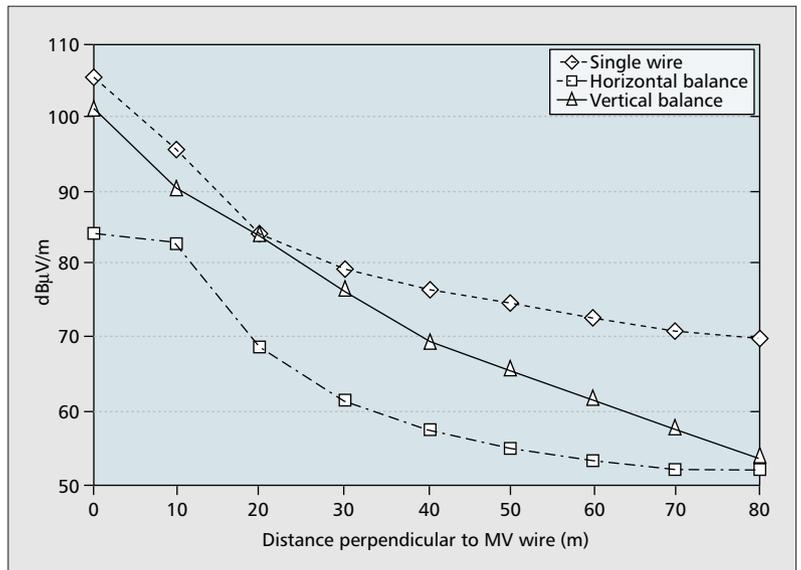
■ Figure 6. Near fields at 20 MHz (2 m above street level) for 1 W signal power.
